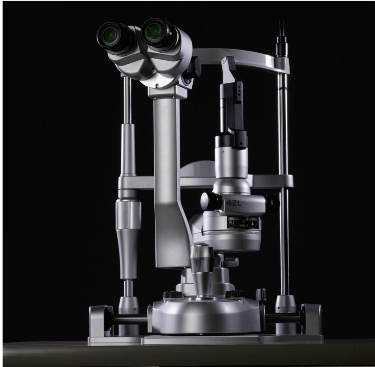
4ZL: High-performance high-grade slit lamp with a 5-step magnification changer, a powerful all-rounder offering total application flexibility
