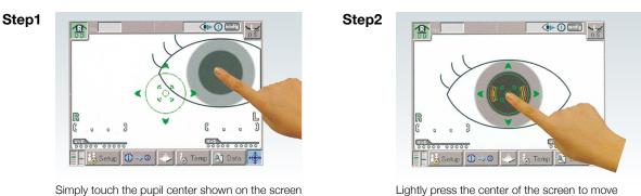
Lightly press the center of the screen to move the measuring head toward the patient. The auto alignment and auto shot functions will then quickly complete measurement.
